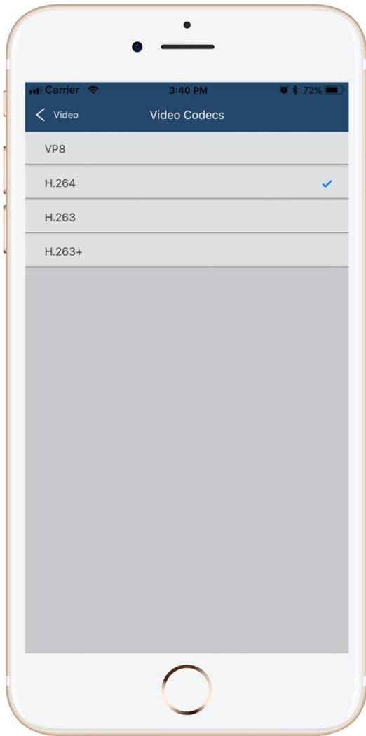
CooCall supports H.263, H.263+, H.264 and VP8 video codecs, by default H.264 has been used. Changing video codecs here also requires changing the same codecs on the IP phone system. And the other party also needs to use the same codecs so a video call can successfully be established.
