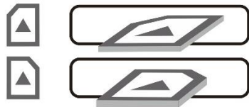
Figure 3-3 Installing a SIM Card
